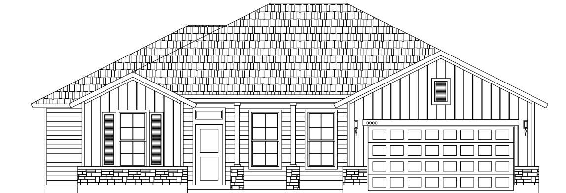
ELEVATION W STONE UPGRADE
